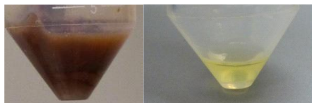
Figure 3: Milk chocolate homogenized in 1-bromonaphthalene (left) and after filtration (right).
