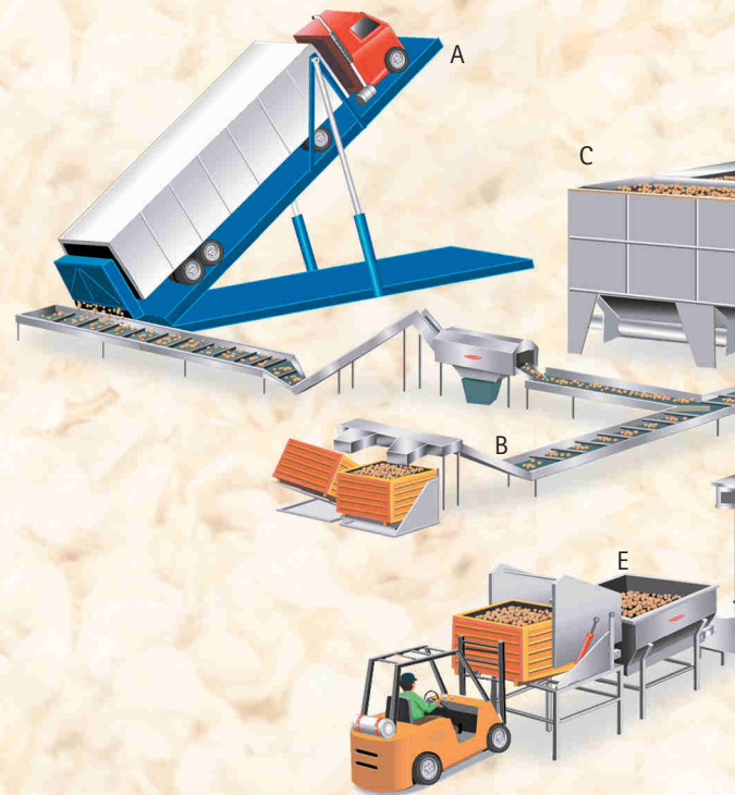
Truck dumping system
