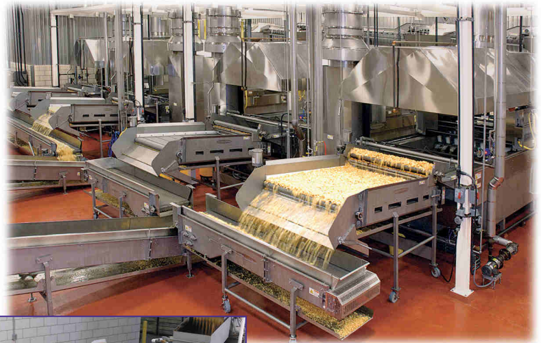
Batch fryers automatically produce popular kettle-style potato chips.
