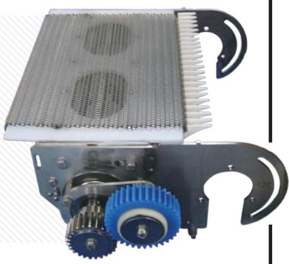
Our Transpositor *provides right-angle product transfers* and allow product lanes or patterns to be built across the width of receiving conveyors. The transfer function uses our sprocket-driven Microspan Chain. Servo or AC motor can power the depositing function.
