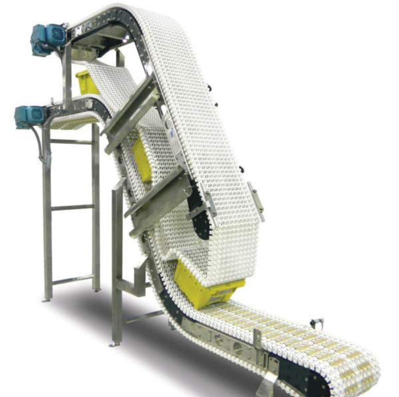
Tackle tricky angles, product orientation and elevation change with a *smaller footprint*. The topper lift puts steep angles within your reach.
