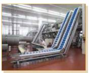
spills and product fall-back. Heavy-duty construction assures trouble-free operation and easy cleaning.
