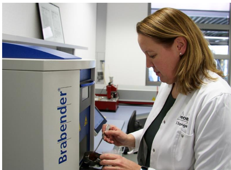
Fig. 4: Sandra Bongers performing one of the only manual steps of moisture analysis with the Brabender MT-CA.
