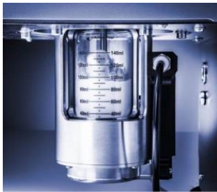
Figure 1: The powder flow cell mounted on an Anton Paar rheometer
