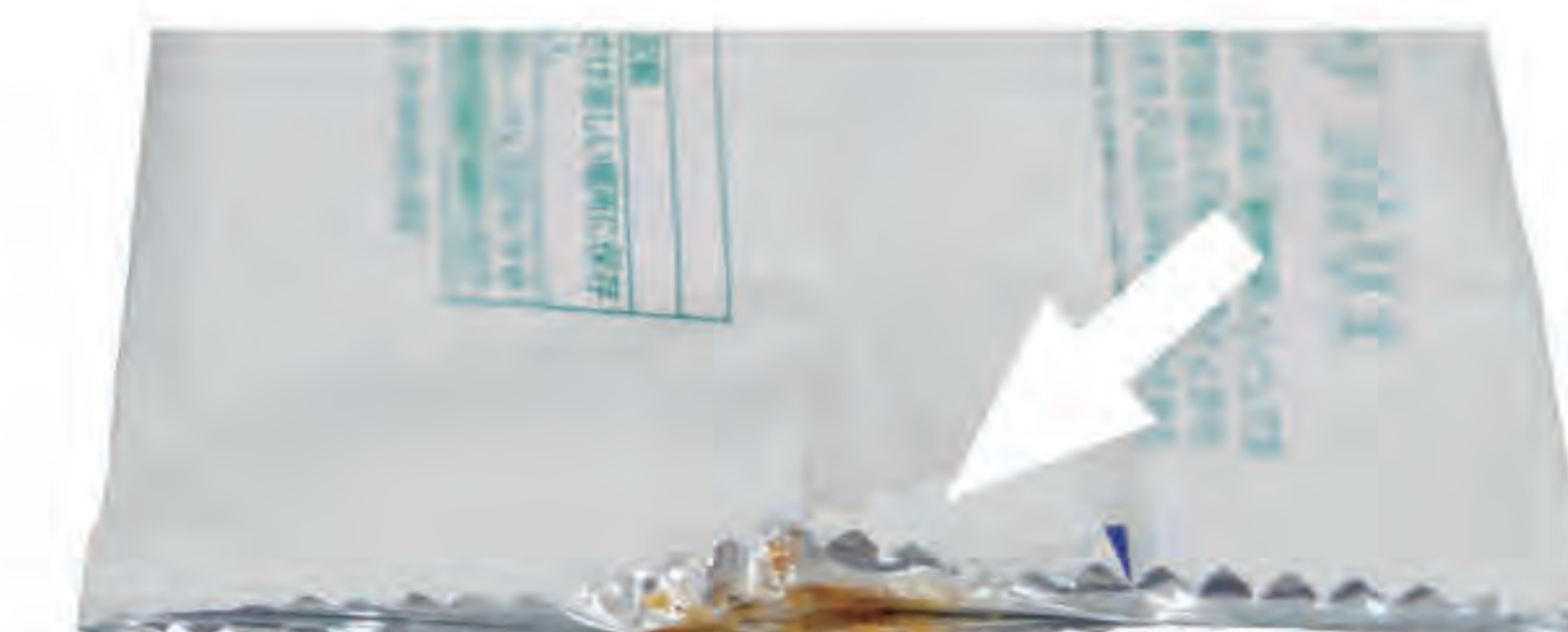
Example of jam inspection of individually-packaged thin product
